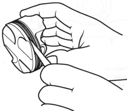
Piston Ring to Ring Groove Clearance Check
